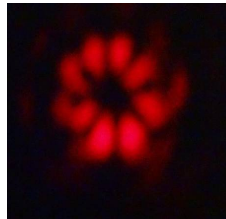
Interference of two optical vortices with m=4 and m=-4 .
